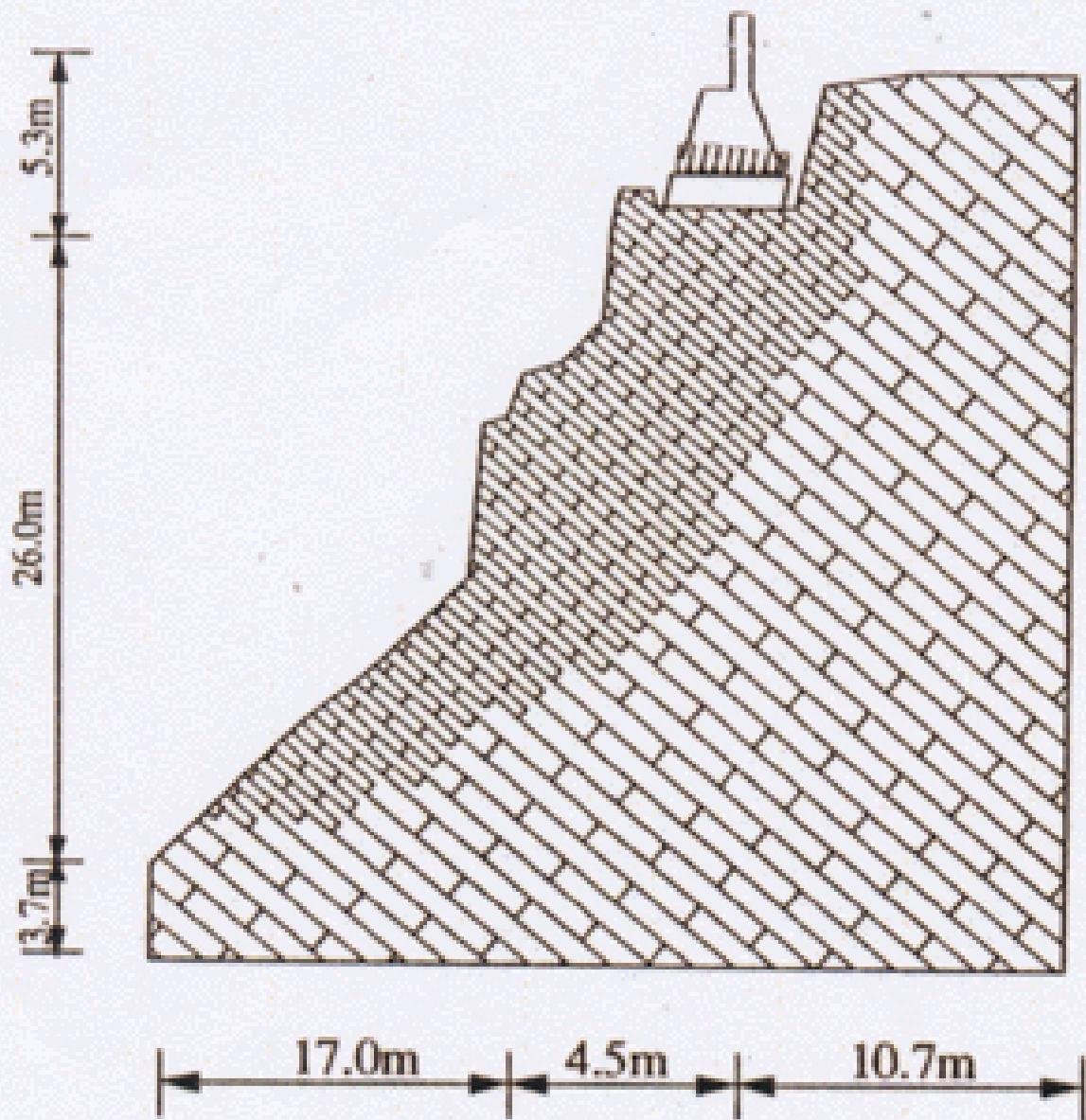
Generation and progress of cracks in the discontinuous rock foundation due to loading
