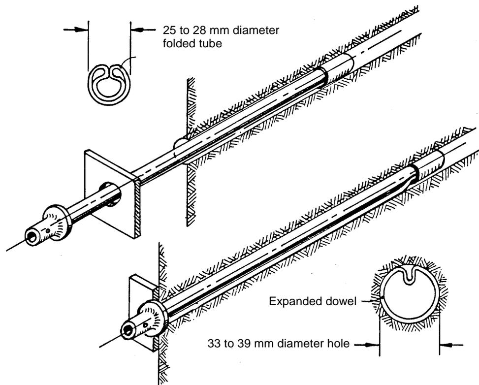
Figure 12.8: Atlas Copco 'Swellex' dowel.
