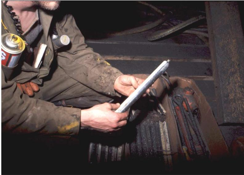
Figure 14.3: Typical two-component resin cartridge used for anchoring and grouting rockbolts.
