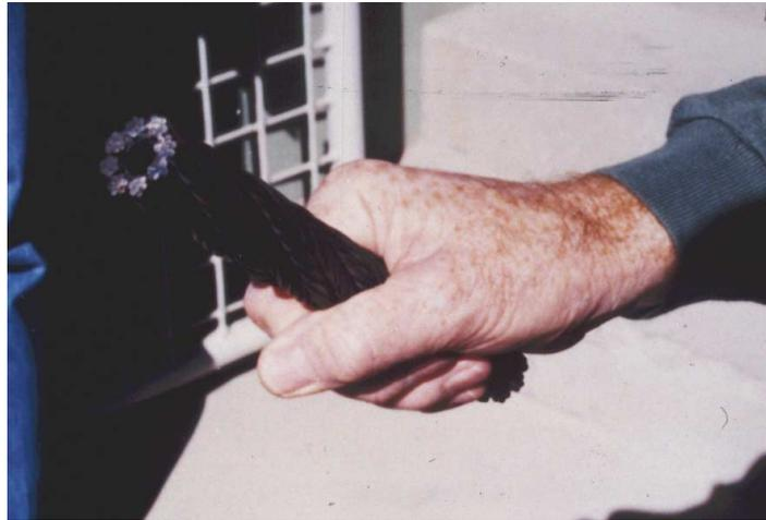
Figure 14.15: Hollow cable by Atlas Copco.
