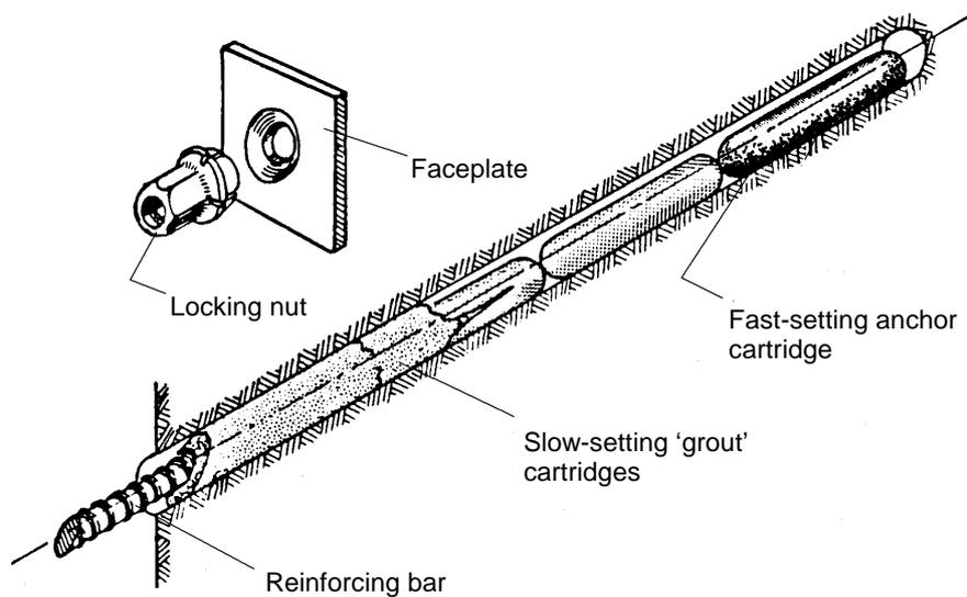
Figure 14.4: Typical set-up for creating a resin anchored and grouted rockbolt. Resin grouting involves placing slow-setting resin cartridges behind the fast-setting anchor cartridges and spinning the bolt rod through them all to mix the resin and catalyst. The bolt is tensioned after the fast-setting anchor resin has set and the slow-setting resin sets later to grout the rod in place.
