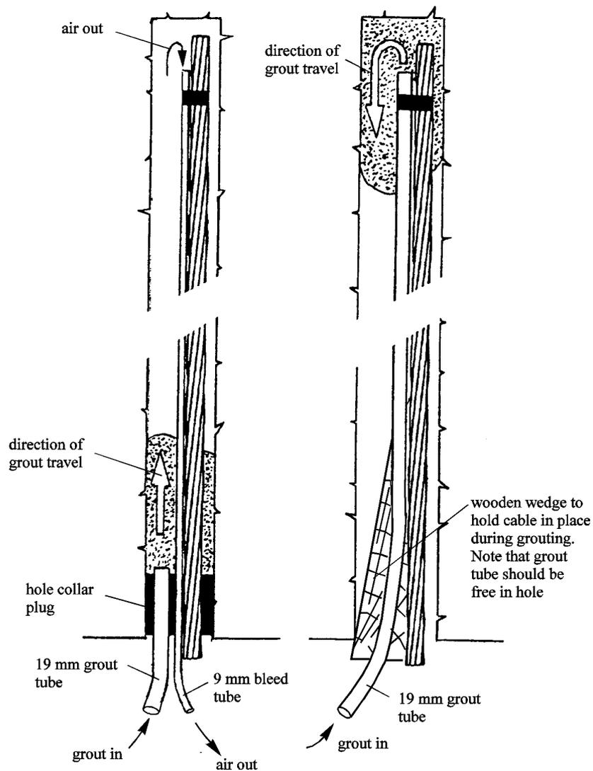
Figure 14.14: Alternative methods for grouting cables in upholes.
