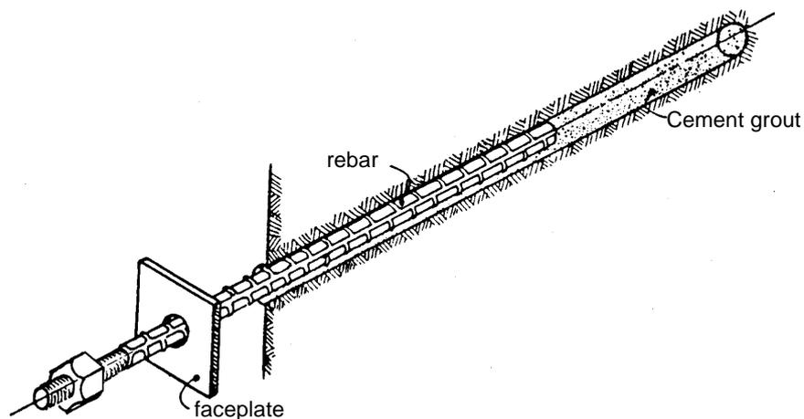
Figure 14.5: Grouted dowel using a deformed bar inserted into a grout-filled hole.
