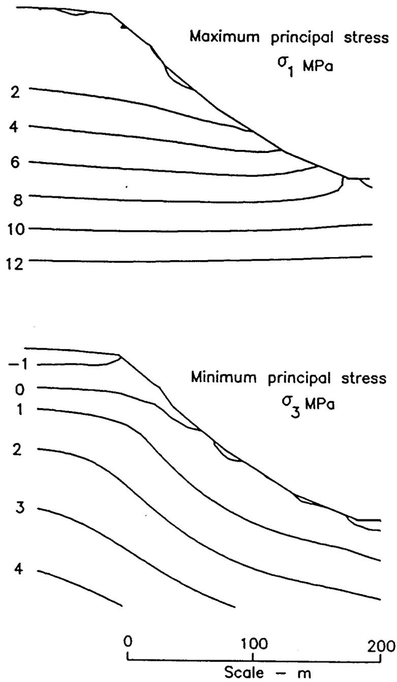
Figure 13.2: Distribution of maximum and minimum principal stresses in a gravitationally loaded slope with far field in situ stresses defined by a ratio of horizontal to vertical stress of 3:1
