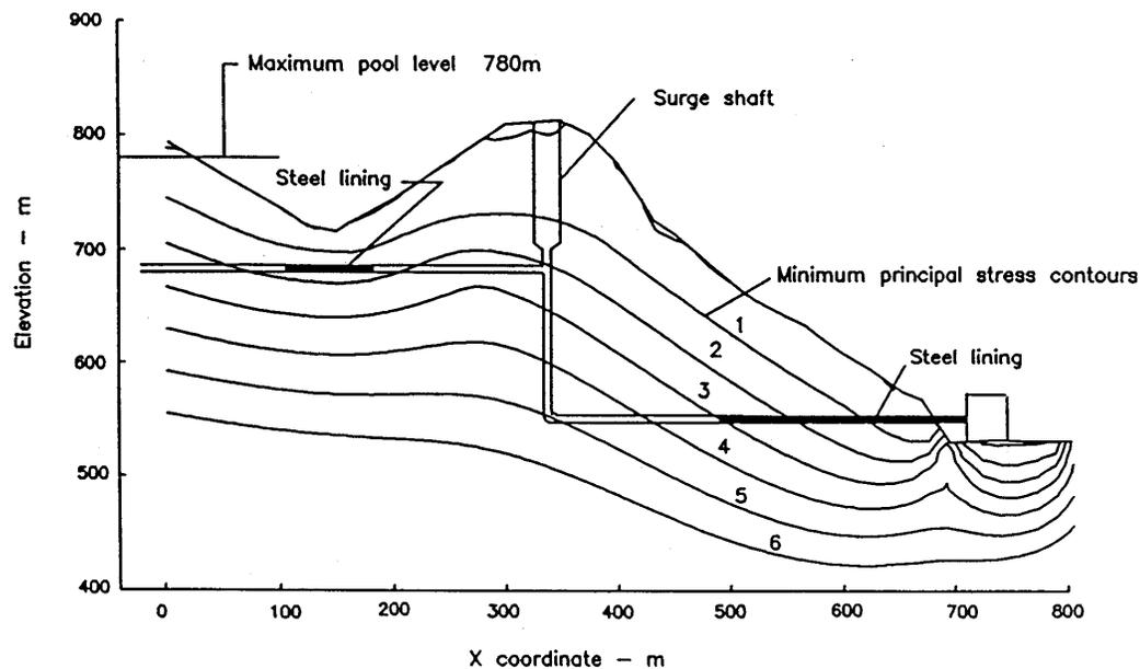
Figure 13.4: Contours of minimum principal stress  $\sigma_3$  (MPa) in a gravitationally loaded slope with a far field in situ stress field defined by a ratio of horizontal to vertical stress of 1.5 : 1. Lengths of steel lining required in the pressure tunnel are shown.
