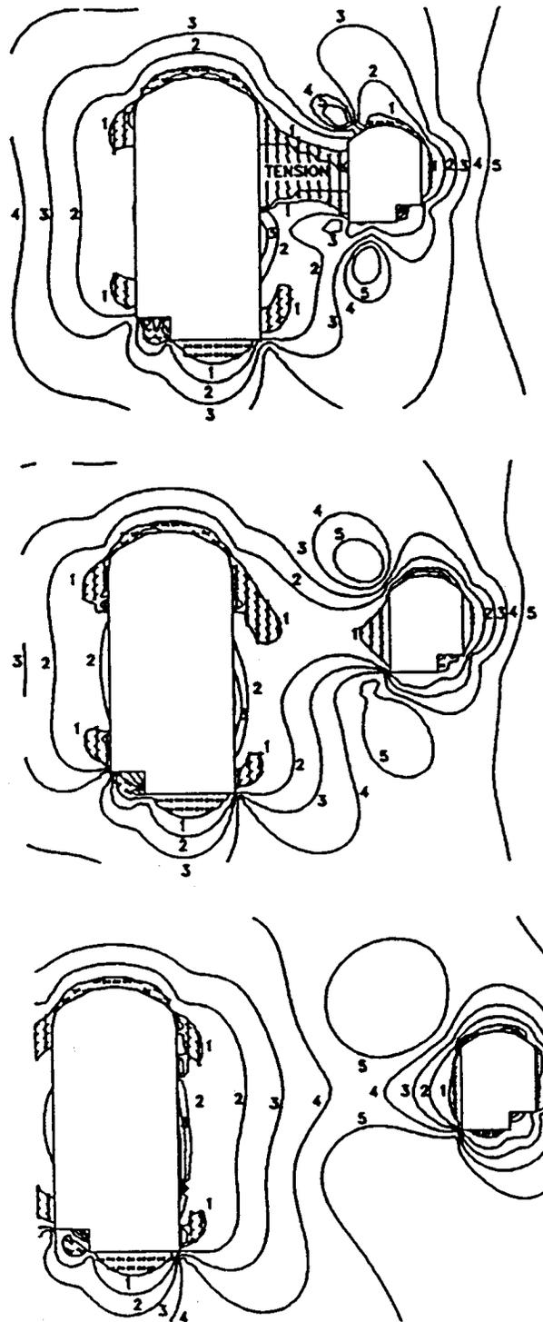
Figure 13.5: Contours of strength/stress ratios and failure trajectories in the rock mass surrounding two adjacent caverns in a siltstone rock mass with different spacing between the caverns.
