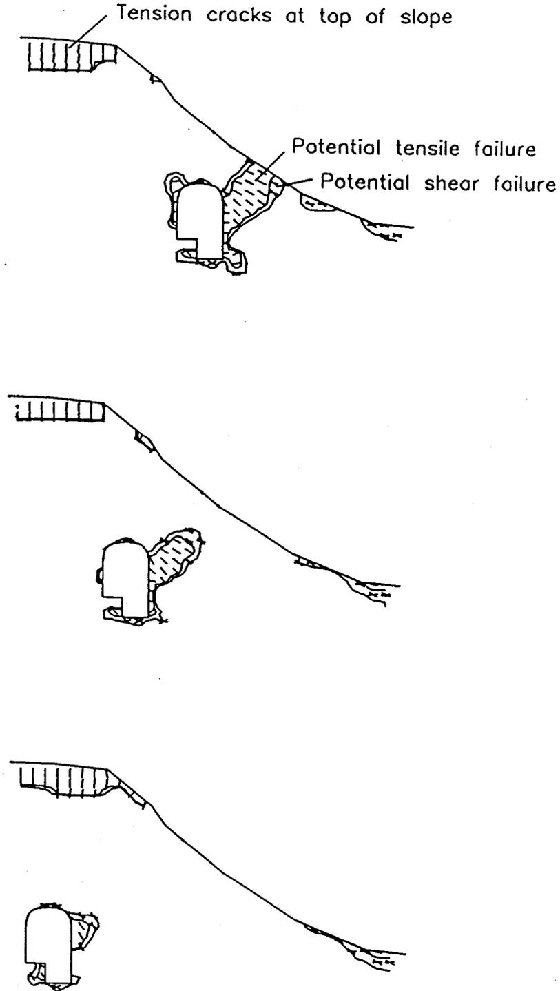
Figure 13.3: Zones of overstress and failure trajectories for a siltstone rock mass surrounding an underground cavern at different distances from the toe of the slope.
