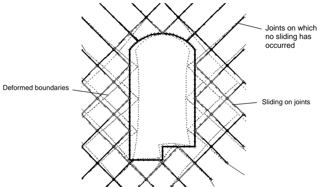
Figure 13.13: Influence of two sets of joints, inclined at  $45^\circ$ , on the displacements on the rock mass surrounding a conventional cavern. The rock mass properties and the in situ stresses are the same as those assumed in the previous section. The joints have a cohesive strength of 0.2 MPa and a friction angle of  $30^\circ$ .
