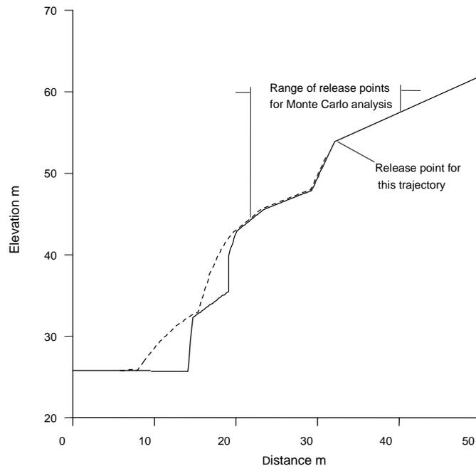
a) Typical trajectory for a 1000 kg boulder.
